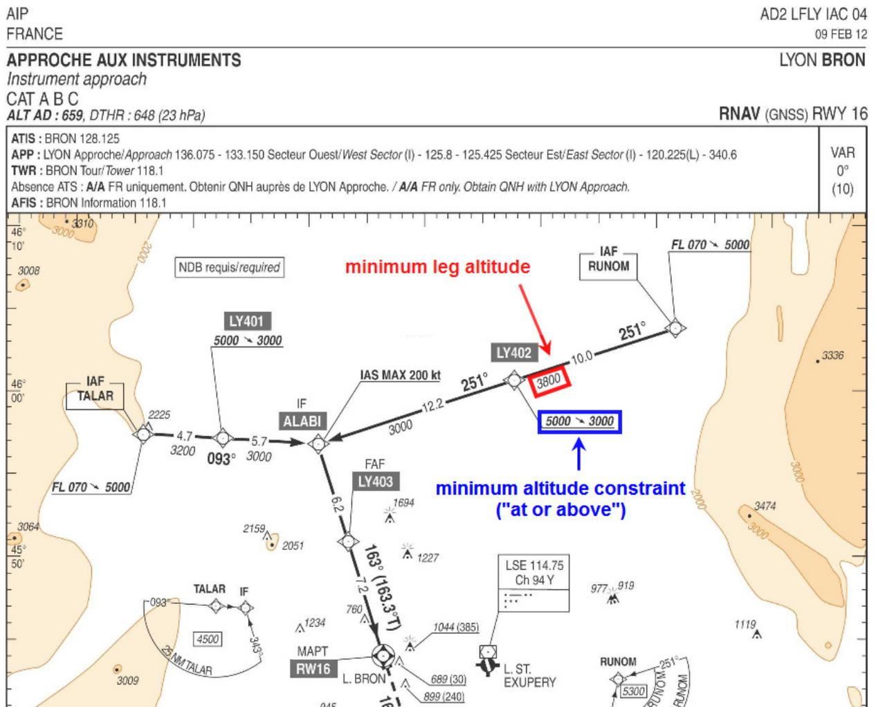
**Fig2: LFLY, RNAV (GNSS) RWY 16, RUNOM transition**
